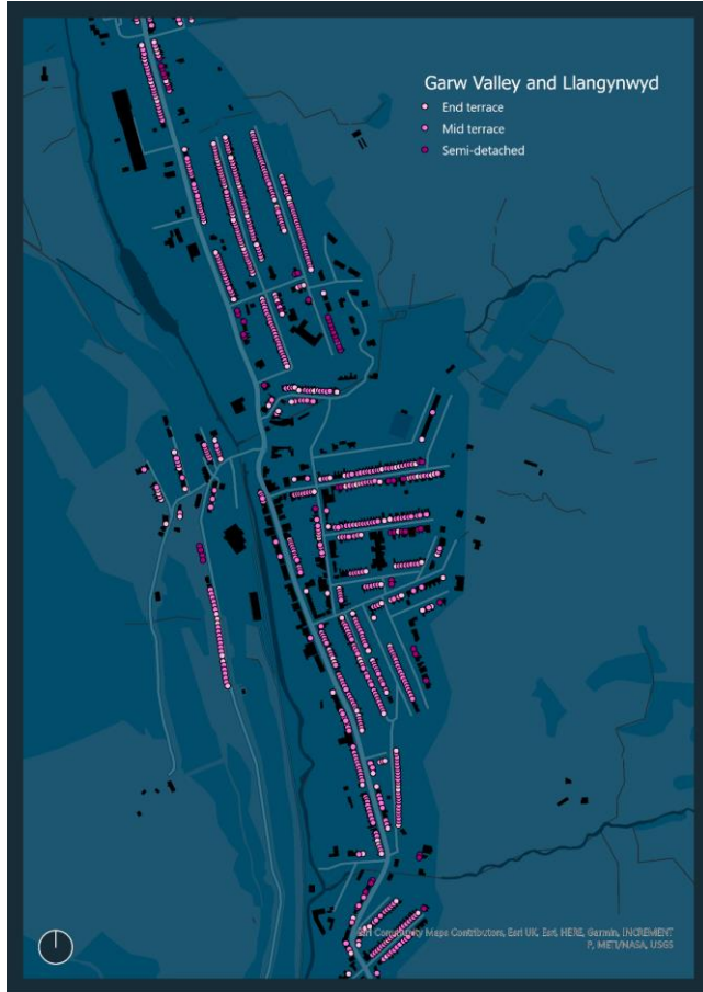
Deep Retrofit Zone 1 – Garw Valley & Llangynwyd A total of 1,100 dwellings requiring deep retrofit fairly evenly split between end-terrace (400), mid-terrace (350), and semi-detached (325) dwellings. The image above shows dwellings in the Pontycymer area which are likely to require a deep retrofit.
