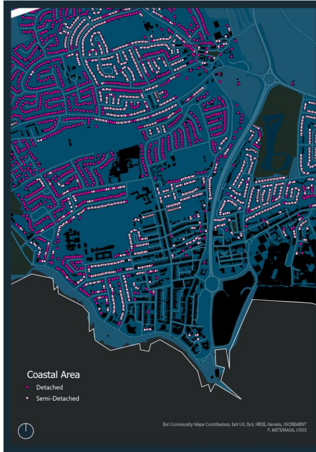
Basic Retrofit Zone 2 – Coastal Area A total of 4,100 dwellings requiring basic retrofit including 1,200 semi-detached and 2,400 detached. The majority of these were constructed between 1945 and 1979. The image above shows dwellings in the Porthcawl and Nottage areas which are likely to require a basic retrofit.
